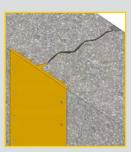
Kryton's Crack Inducing Waterstop creates a controlled crack and then introduces Krystol technology through an externally placed waterstop that ensures permanent waterproofing protection.
