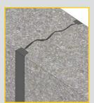
Aligned keyways create a controlled crack to introduce Krystol technology through two external waterstops that ensure permanent waterproofing protection.
